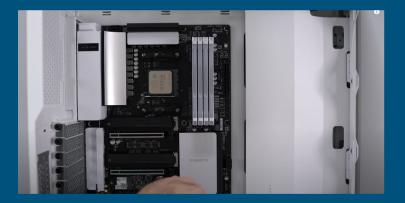
Step 4: Screwing the motherboard into the case
